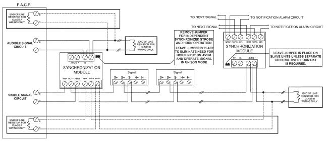
Note: See Technical Bulletin 015 for proper synchronization module for application. Note: When synchronizing the GEH-12 VDC Series, the AVSM synchronization module <u>MUST</u> be used.
